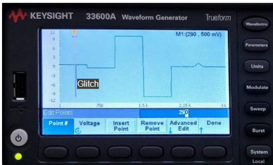
Figure 2. Edit a single point to create a glitch in the test signal
