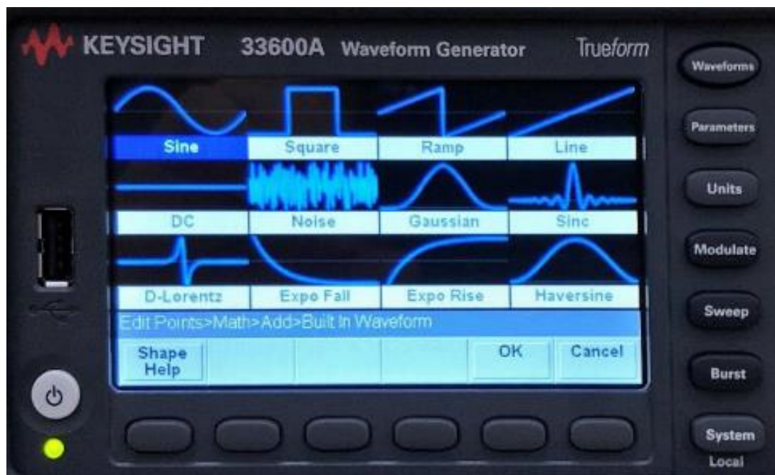
Figure 3. Build-in waveforms shown are sine, square, ramp, line, DC, noise, Gaussian, sinc, Lorentz, fall and rise, and haversine
