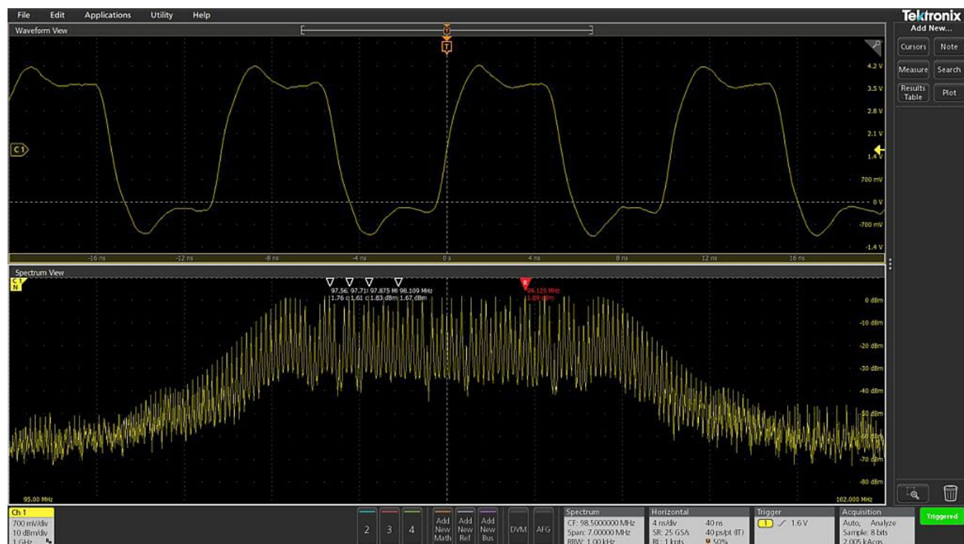
FIGURE 5. Looking at the same spread-spectrum clock signal as Figures 3 and 4, Spectrum View enables optimized views of both time and frequency domains at the same time.
