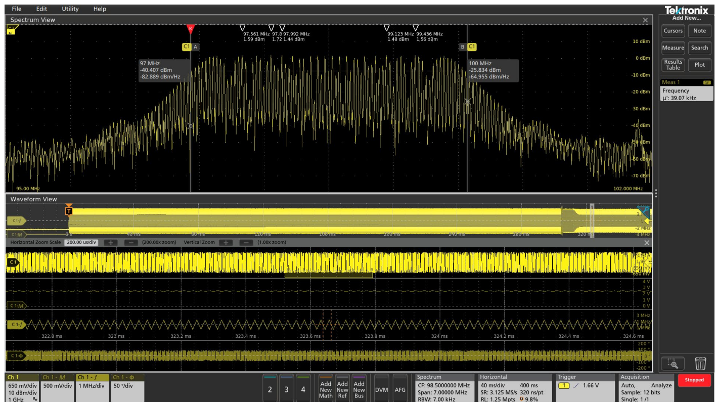
FIGURE 12. We've now zoomed in even further and can easily view the triangular frequency modulation in use and can confirm through the automatic measurement in the results bar that we are getting the correct modulation rate of 39.07 kHz.
