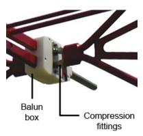
Align the compression fittings with the threaded connectors on the balun box.
