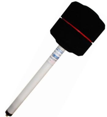
The radiation pattern is omni directional in the H plane, allowing the antenna to receive signals from every direction around the axis. The range covers most wireless bands worldwide, and is designed for the lowest possible VSWR across the range of operation. The antenna exhibits better than 2:1 VSWR for most of the range, and never exceeds 5:1 above 1 GHz.
