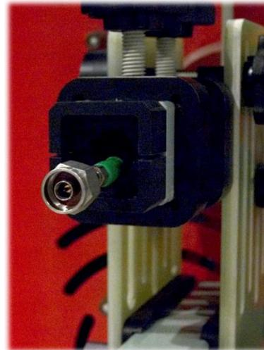
2. Attach the cable to the Type N connector at the end of the stinger.
